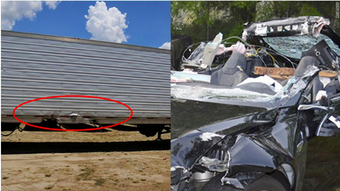
Tesla autopilot failed to recognize a white truck against bright sky leading to fatal crash
